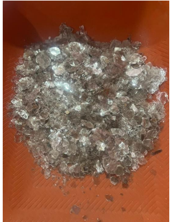
Figure 7. Mica flakes made from dhibra or crude mica. Photo courtesy of RMI
