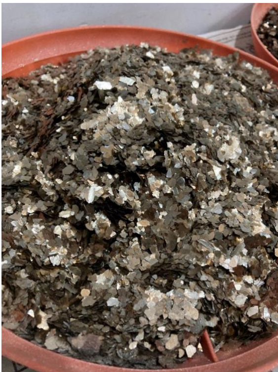
Figure 8. Calcined mica. Photo courtesy of RMI
