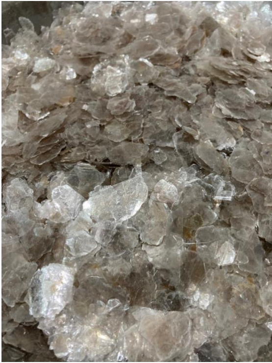
Figure 6. High-quality mica scrap. Photo courtesy of RMI
