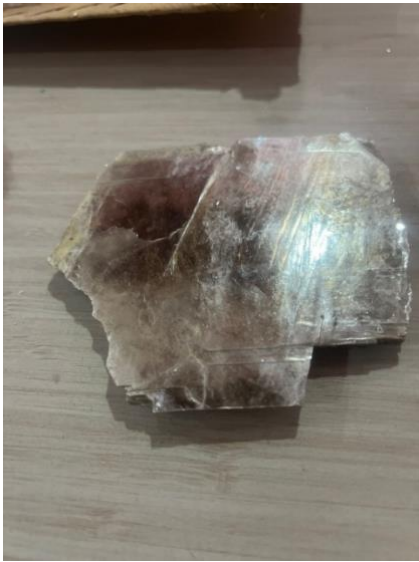
Figure 2. Images of book mica, from which mica films, splittings, and thins are cobbled by hand. Image courtesy of RMI
