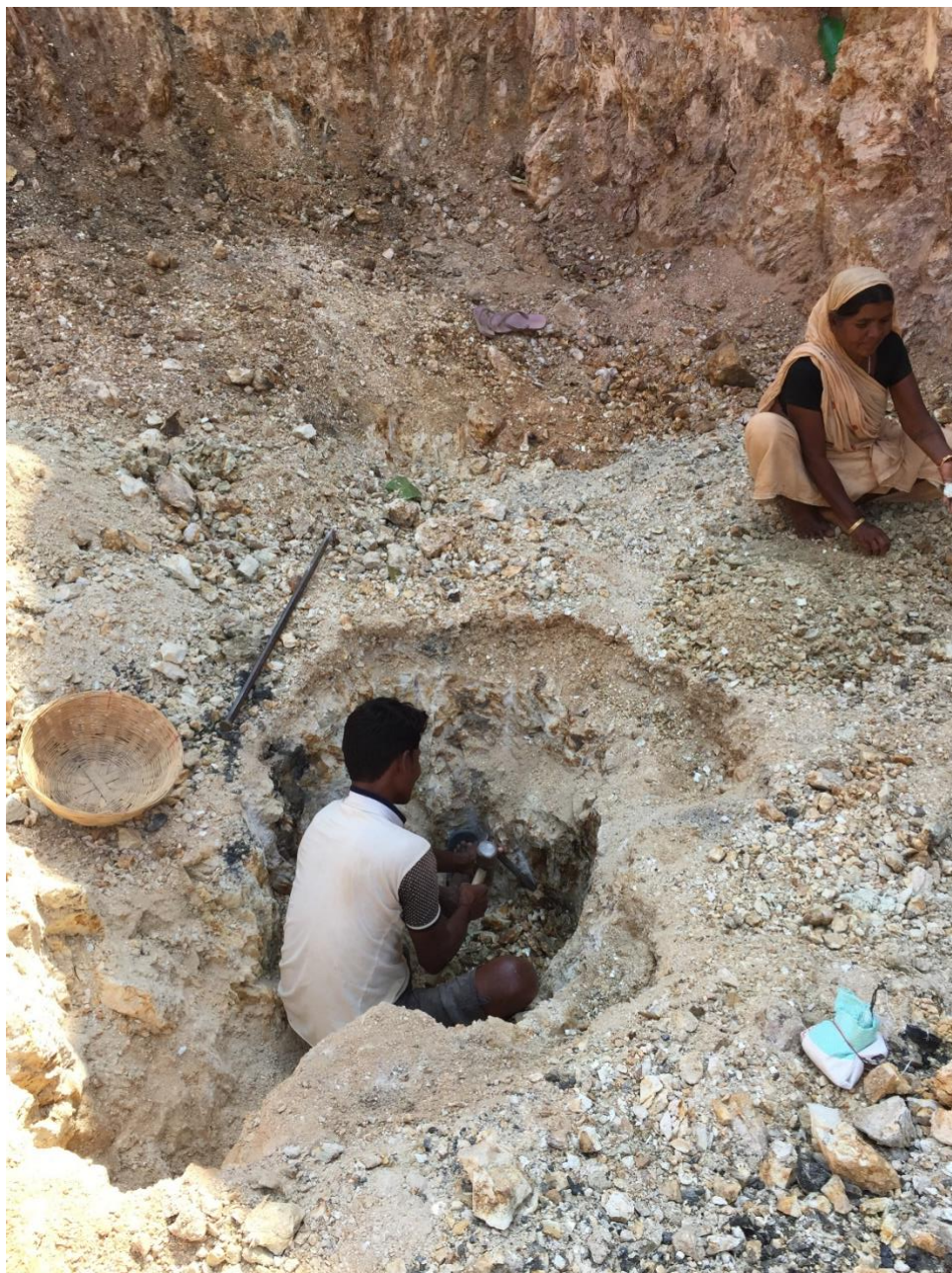
Figure 4. Hammering away to release mica books (left) and sorting through piles of debris/ dhibra (right). Photo courtesy of RMI
