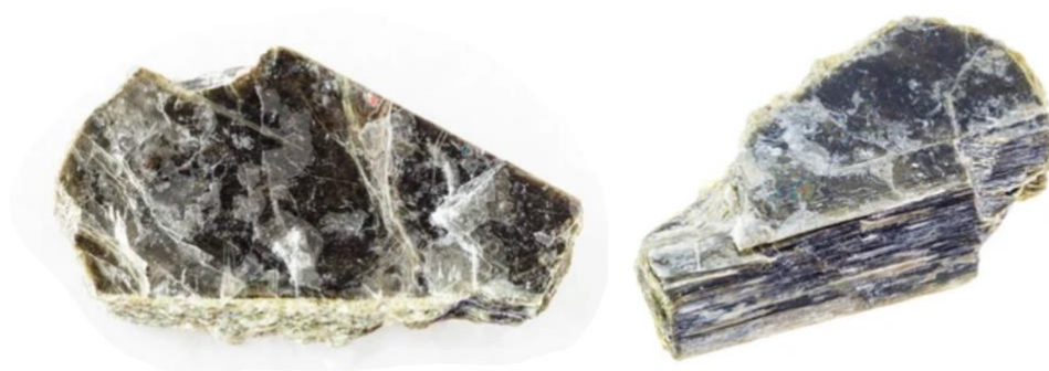
Figure 1. Images of book mica, from which mica splittings and thins are cobbled by hand 30
