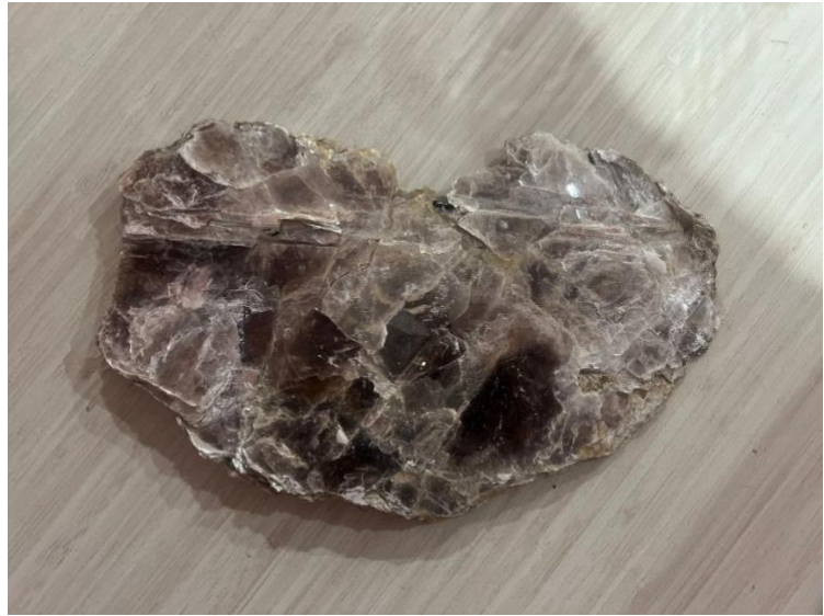
Figure 2. Images of book mica, from which mica films, splittings, and thins are cobbled by hand. Image courtesy of RMI
