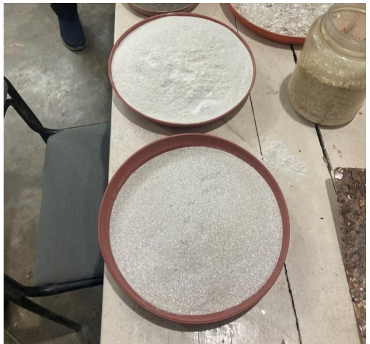
Figure 9. Different types of mica powder (calcined at top, ordinary at bottom). Photo courtesy of RMI
