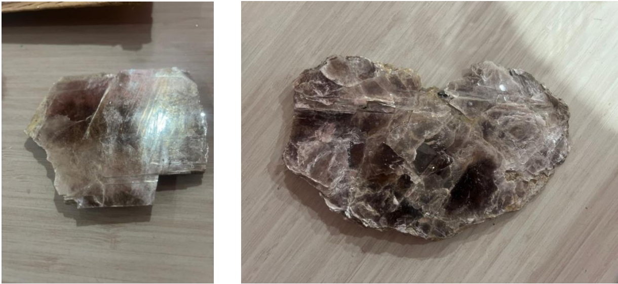
Figure 2. Images of book mica, from which mica films, splittings, and thins are cobbled by hand. Image courtesy of RMI
