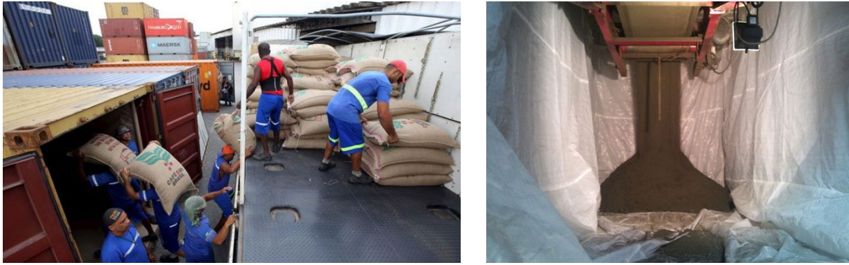
Figure 16. On the left, a container full of 60 kg bags of coffee is loaded at the port. On the right, a hermetically sealed container full of coffee in bulk. Sources:
